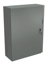
Wiegmann Ultimate series disconnect enclosure, NEMA 4/12/13, right flange,  $42 \times 32 \times 12$  in (HxWxD), wall mount, carbon steel, ANSI 61 gray, powder coat finish, single-door, 3-point padlocking handle, purchase subpanel separately.
