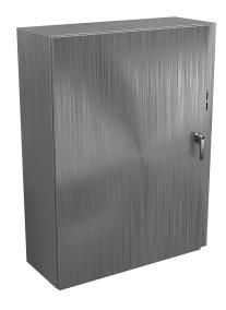
Wiegmann Ultimate series disconnect enclosure, NEMA 4/4X/12/13, right flange, 42 x 32 x 12in (HxWxD), wall mount, 316L stainless steel, No. 3 intermediate polished finish, singledoor, 3-point padlocking handle, purchase subpanel separately.
