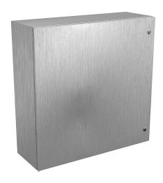
Wiegmann Ultimate series enclosure, NEMA 4/4X/12/13, 36 x 36 x 12in (HxWxD), wall mount, 304 stainless steel, No. 3 intermediate polished finish, single-door, 1/4-turn semi-flush oil-tight latch.
