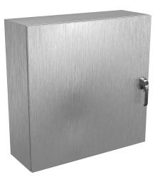
Wiegmann Ultimate series enclosure, NEMA 4X/12/13, 36 x 36 x 12in (HxWxD), wall mount, 304 stainless steel, No. 3 intermediate polished finish, single-door, 3-point 316L padlocking handle.
