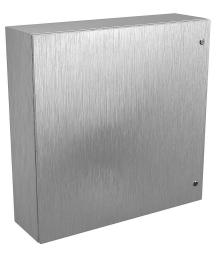
Wiegmann Ultimate series enclosure, NEMA 4/4X/12/13,  $36 \times 36 \times 10$  in (HxWxD), wall mount, 304 stainless steel, No. 3 intermediate polished finish, single-door, 1/4-turn semi-flush oil-tight latch.
