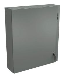
Wiegmann Ultimate series disconnect enclosure, NEMA 4/12/13, right flange, 36 x 32 x 8in (HxWxD), wall mount, carbon steel, ANSI 61 gray, powder coat finish, single-door, 2-point padlocking handle, purchase subpanel separately.
