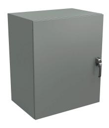
Wiegmann Ultimate series enclosure, NEMA 4/12/13, 36 x 30 x 20in (HxWxD), wall mount, carbon steel, ANSI 61 gray, powder coat finish, single-door, 3-point keylocking/padlocking combo handle.
