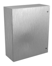
Wiegmann Ultimate series enclosure, NEMA 4/4X/12/13, 36 x 30 x 12in (HxWxD), wall mount, 304 stainless steel, No. 3 intermediate polished finish, single-door, 1/4-turn semi-flush oil-tight latch.
