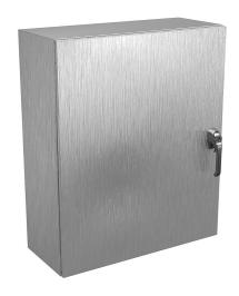
Wiegmann Ultimate series enclosure, NEMA 4X/12/13,  $36 \times 30 \times 12$  in (HxWxD), wall mount, 304 stainless steel, No. 3 intermediate polished finish, single-door, 3-point 316L padlocking handle.
