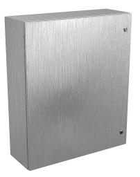
Wiegmann Ultimate series enclosure, NEMA 4/4X/12/13, 36 x 30 x 10in (HxWxD), wall mount, 304 stainless steel, No. 3 intermediate polished finish, single-door, 1/4-turn semi-flush oil-tight latch.
