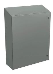
Wiegmann Ultimate series enclosure, slope top, NEMA 4/12/13, 36 x 30 x 10in (HxWxD), wall mount, carbon steel, ANSI 61 gray, powder coat finish, single-door, 1/4-turn semi-flush oil-tight latch.
