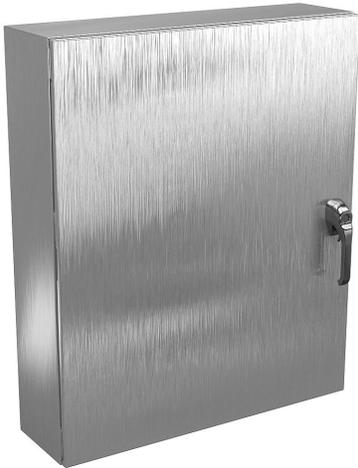
Wiegmann Ultimate series enclosure, NEMA 4X/12/13, 36 x 30 x 8in (HxWxD), wall mount, 304 stainless steel, No. 3 intermediate polished finish, single-door, 3-point 316L padlocking handle.
