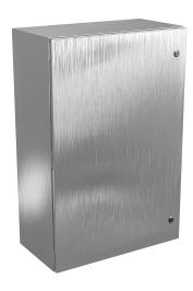
Wiegmann Ultimate series enclosure, NEMA 4/4X/12/13, 36 x 24 x 12in (HxWxD), wall mount, 304 stainless steel, No. 3 intermediate polished finish, single-door, 1/4-turn semi-flush oil-tight latch.
