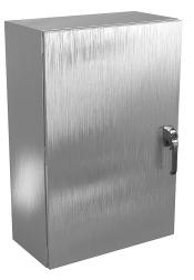
Wiegmann Ultimate series enclosure, NEMA 4X/12/13, 36 x 24 x 12in (HxWxD), wall mount, 304 stainless steel, No. 3 intermediate polished finish, single-door, 3-point 316L padlocking handle.
