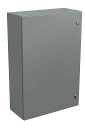
Wiegmann Ultimate series enclosure, NEMA 4/12/13, 36 x 24 x 10in (HxWxD), wall mount, carbon steel, ANSI 61 gray, powder coat finish, single-door, 1/4-turn semi-flush oil-tight latch.
