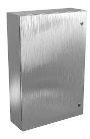
Wiegmann Ultimate series enclosure, NEMA 4/4X/12/13, 36 x 24 x 8in (HxWxD), wall mount, 304 stainless steel, No. 3 intermediate polished finish, single-door, 1/4-turn semi-flush oil-tight latch.
