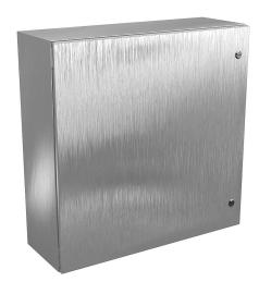
Wiegmann Ultimate series enclosure, NEMA 4/4X/12/13,  $30 \times 30 \times 10$  in (HxWxD), wall mount, 316L stainless steel, No. 3 intermediate polished finish, single-door, 1/4-turn semi-flush oil-tight latch.
