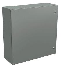
Wiegmann Ultimate series enclosure, NEMA 4/12/13, 30 x 30 x 10in (HxWxD), wall mount, carbon steel, ANSI 61 gray, powder coat finish, single-door, 1/4-turn semi-flush oil-tight latch.
