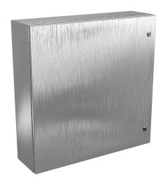
Wiegmann Ultimate series enclosure, NEMA 4/4X/12/13,  $30 \times 30 \times 8$ in (HxWxD), wall mount, 304 stainless steel, No. 3 intermediate polished finish, single-door, 1/4-turn semi-flush oil-tight latch.
