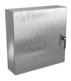
Wiegmann Ultimate series enclosure, NEMA 4X/12/13,  $30 \times 30 \times 8$  in (HxWxD), wall mount, 304 stainless steel, No. 3 intermediate polished finish, single-door, 3-point 316L padlocking handle.
