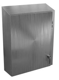
Wiegmann Ultimate series disconnect enclosure, slope top, NEMA 4/4X/12/13, right flange, 30 x 26 x 8in (HxWxD), wall mount, 304 stainless steel, No. 3 intermediate polished finish, single-door, 2-point padlocking handle, purchase subpanel separately.
