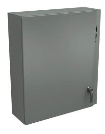
Wiegmann Ultimate series disconnect enclosure, NEMA 4/12/13, right flange, 30 x 26 x 8in (HxWxD), wall mount, carbon steel, ANSI 61 gray, powder coat finish, single-door, 2-point padlocking handle, purchase subpanel separately.
