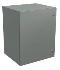
Wiegmann Ultimate series enclosure, NEMA 4/12/13, 30 x 24 x 20in (HxWxD), wall mount, carbon steel, ANSI 61 gray, powder coat finish, single-door, 1/4-turn semi-flush oil-tight latch.
