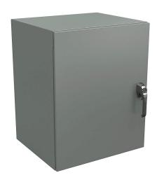
Wiegmann Ultimate series enclosure, NEMA 4/12/13, 30 x 24 x 20in (HxWxD), wall mount, carbon steel, ANSI 61 gray, powder coat finish, single-door, 3-point keylocking/padlocking combo handle.
