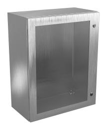
Wiegmann Ultimate series enclosure, NEMA 4/4X/12/13, 30 x 24 x 12in (HxWxD), wall mount, 304 stainless steel, No. 3 intermediate polished finish, single-door, 1/4-turn semi-flush oil-tight latch, polycarbonate window.
