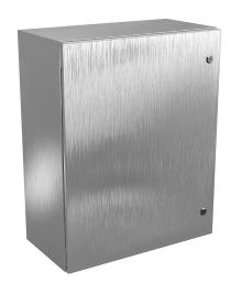
Wiegmann Ultimate series enclosure, NEMA 4/4X/12/13, 30 x 24 x 12in (HxWxD), wall mount, 304 stainless steel, No. 3 intermediate polished finish, single-door, 1/4-turn semi-flush oil-tight latch.
