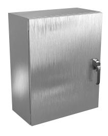
Wiegmann Ultimate series enclosure, NEMA 4X/12/13, 30 x 24 x 12in (HxWxD), wall mount, 304 stainless steel, No. 3 intermediate polished finish, single-door, 3-point 316L padlocking handle.
