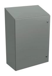
Wiegmann Ultimate series enclosure, slope top, NEMA 4/12/13,  $30 \times 24 \times 12$ in (HxWxD), wall mount, carbon steel, ANSI 61 gray, powder coat finish, single-door, 1/4-turn semi-flush oil-tight latch.
