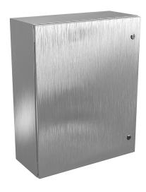
Wiegmann Ultimate series enclosure, NEMA 4/4X/12/13,  $30 \times 24 \times 10$  in (HxWxD), wall mount, 304 stainless steel, No. 3 intermediate polished finish, single-door, 1/4-turn semi-flush oil-tight latch.
