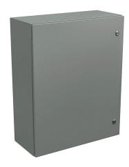
Wiegmann Ultimate series enclosure, NEMA 4/12/13, 30 x 24 x 10in (HxWxD), wall mount, carbon steel, ANSI 61 gray, powder coat finish, single-door, 1/4-turn semi-flush oil-tight latch.
