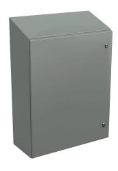
Wiegmann Ultimate series enclosure, slope top, NEMA 4/12/13,  $30 \times 24 \times 10$  in (HxWxD), wall mount, carbon steel, ANSI 61 gray, powder coat finish, single-door, 1/4-turn semi-flush oil-tight latch.
