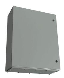
Wiegmann Ultimate series enclosure, NEMA 3R/4/12/13, 30 x 24 x 10in (HxWxD), wall mount, bottom gland plate, carbon steel, ANSI 61 gray, powder coat finish, single-door, 1/4-turn semi-flush oiltight latch.
