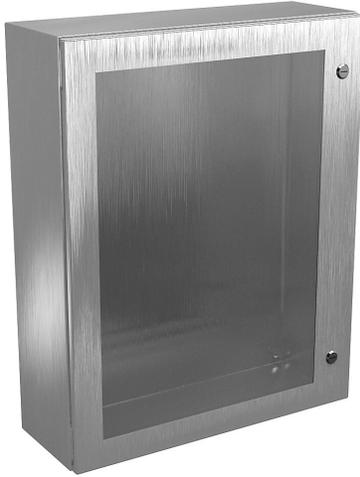
Wiegmann Ultimate series enclosure, NEMA 4/4X/12/13, 30 x 24 x 8in (HxWxD), wall mount, 304 stainless steel, No. 3 intermediate polished finish, single-door, 1/4-turn semi-flush oil-tight latch, polycarbonate window.
