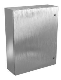
Wiegmann Ultimate series enclosure, NEMA 4/4X/12/13, 30 x 24 x 8in (HxWxD), wall mount, 304 stainless steel, No. 3 intermediate polished finish, single-door, 1/4-turn semi-flush oil-tight latch.
