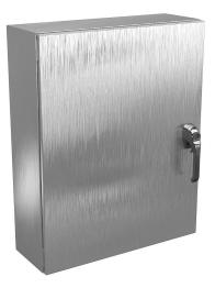
Wiegmann Ultimate series enclosure, NEMA 4X/12/13, 30 x 24 x 8in (HxWxD), wall mount, 304 stainless steel, No. 3 intermediate polished finish, single-door, 3-point 316L padlocking handle.
