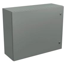
Wiegmann Ultimate series enclosure, NEMA 4/12/13, 24 x 30 x 10in (HxWxD), wall mount, carbon steel, ANSI 61 gray, powder coat finish, single-door, 1/4-turn semi-flush oil-tight latch.
