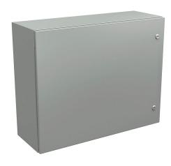
Wiegmann Ultimate series enclosure, NEMA 4/12/13,  $24 \times 30 \times 10$  in (HxWxD), wall mount, carbon steel, RAL 7035 light gray, powder coat finish, single-door, 1/4-turn semi-flush oil-tight latch.
