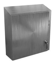
Wiegmann Ultimate series disconnect enclosure, slope top, NEMA 4/4X/12/13, right flange, 24 x 26 x 8in (HxWxD), wall mount, 304 stainless steel, No. 3 intermediate polished finish, singledoor, 2-point padlocking handle, purchase subpanel separately.
