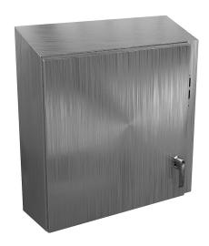
Wiegmann Ultimate series disconnect enclosure, slope top, NEMA 4/4X/12/13, right flange, 24 x 26 x 8in (HxWxD), wall mount, 304 stainless steel, No. 3 intermediate polished finish, singledoor, 2-point padlocking handle, purchase subpanel separately.
