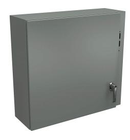
Wiegmann Ultimate series disconnect enclosure, NEMA 4/12/13, right flange, 24 x 26 x 8in (HxWxD), wall mount, carbon steel, ANSI 61 gray, powder coat finish, single-door, 2-point padlocking handle, purchase subpanel separately.
