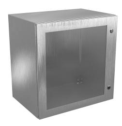
Wiegmann Ultimate series enclosure, NEMA 4/4X/12/13,  $24 \times 24 \times 16$  in (HxWxD), wall mount, 304 stainless steel, No. 3 intermediate polished finish, single-door, 1/4-turn semi-flush oil-tight latch, polycarbonate window.
