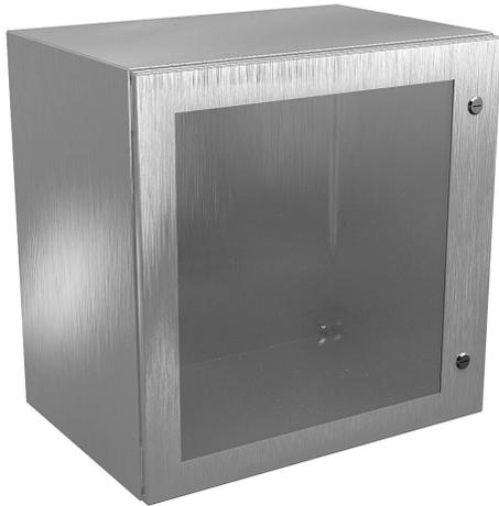
Wiegmann Ultimate series enclosure, NEMA 4/4X/12/13, 24 x 24 x 16in (HxWxD), wall mount, 304 stainless steel, No. 3 intermediate polished finish, single-door, 1/4-turn semi-flush oil-tight latch, polycarbonate window.
