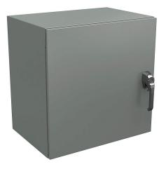
Wiegmann Ultimate series enclosure, NEMA 4/12/13, 24 x 24 x 16in (HxWxD), wall mount, carbon steel, ANSI 61 gray, powder coat finish, single-door, 3-point keylocking/padlocking combo handle.
