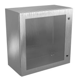
Wiegmann Ultimate series enclosure, NEMA 4/4X/12/13, 24 x 24 x 12in (HxWxD), wall mount, 304 stainless steel, No. 3 intermediate polished finish, single-door, 1/4-turn semi-flush oil-tight latch, polycarbonate window.
