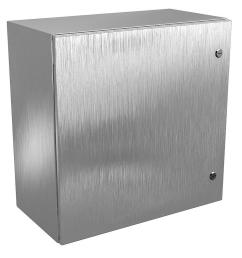
Wiegmann Ultimate series enclosure, NEMA 4/4X/12/13,  $24 \times 24 \times 12$  in (HxWxD), wall mount, 304 stainless steel, No. 3 intermediate polished finish, single-door, 1/4-turn semi-flush oil-tight latch.
