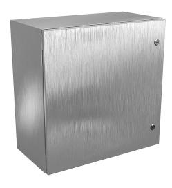
Wiegmann Ultimate series enclosure, NEMA 4/4X/12/13, 24 x 24 x 12in (HxWxD), wall mount, 316L stainless steel, No. 3 intermediate polished finish, single-door, 1/4-turn semi-flush oil-tight latch.
