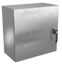
Wiegmann Ultimate series enclosure, NEMA 4X/12/13, 24 x 24 x 12in (HxWxD), wall mount, 304 stainless steel, No. 3 intermediate polished finish, single-door, 3-point 316L padlocking handle.
