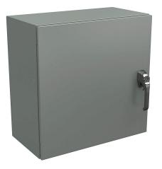
Wiegmann Ultimate series enclosure, NEMA 4/12/13, 24 x 24 x 12in (HxWxD), wall mount, carbon steel, ANSI 61 gray, powder coat finish, single-door, 3-point keylocking/padlocking combo handle.
