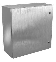
Wiegmann Ultimate series enclosure, NEMA 4/4X/12/13,  $24 \times 24 \times 10$  in (HxWxD), wall mount, 316L stainless steel, No. 3 intermediate polished finish, single-door, 1/4-turn semi-flush oil-tight latch.
