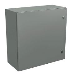
Wiegmann Ultimate series enclosure, NEMA 4/12/13, 24 x 24 x 10in (HxWxD), wall mount, carbon steel, ANSI 61 gray, powder coat finish, single-door, 1/4-turn semi-flush oil-tight latch.
