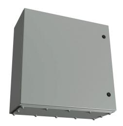
Wiegmann Ultimate series enclosure, NEMA 3R/4/12/13, 24 x 24 x 10in (HxWxD), wall mount, bottom gland plate, carbon steel, ANSI 61 gray, powder coat finish, single-door, 1/4-turn semi-flush oiltight latch.
