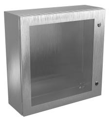
Wiegmann Ultimate series enclosure, NEMA 4/4X/12/13, 24 x 24 x 8in (HxWxD), wall mount, 304 stainless steel, No. 3 intermediate polished finish, single-door, 1/4-turn semi-flush oil-tight latch, polycarbonate window.
